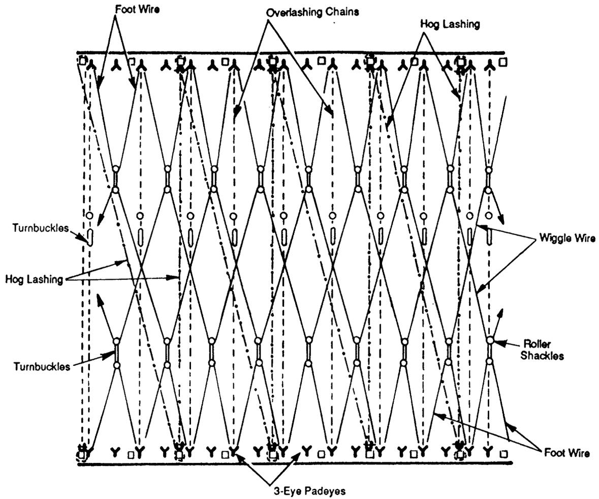
**NOTE:** *Roler Shackles to be affixed between all Foot Wires and Wiggle Wires and at least two Turnbuckles to be inserted between the Wiggle Wire and the Foot Wire on each side (Port and Starboard)*
